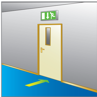
At each exit door
